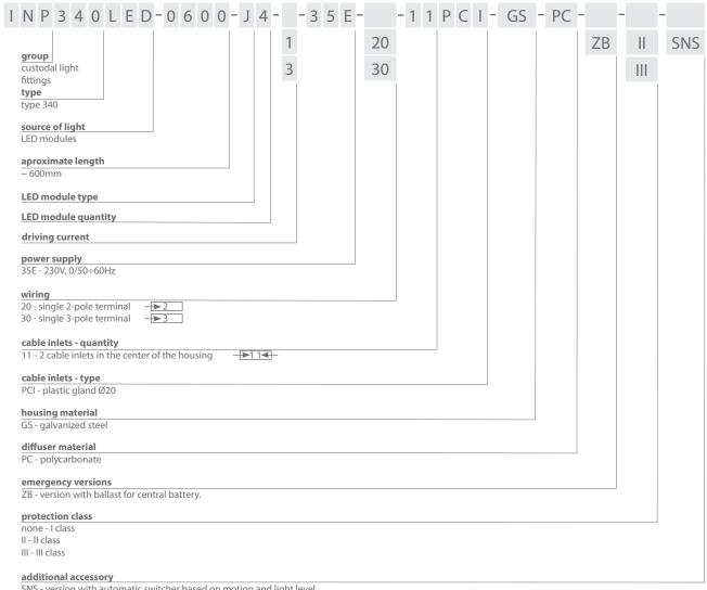
SNS - version with automatic switcher based on motion and light level.
