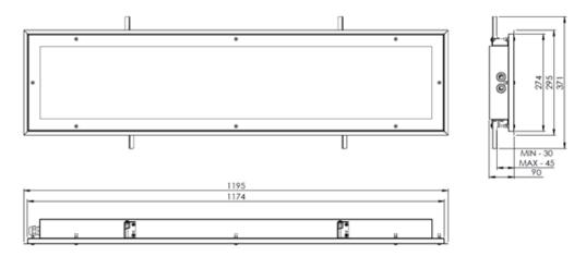
EXF390LED-1200-FA2 and EXF390LED-1200-FA4, mounting directly on the ceiling:
