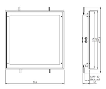
EXF390LED-0600-FA4, mounting directly on the ceiling:
