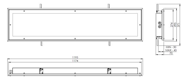
EXL390LED-1200-E3 and EXL390LED-1200-E6, mounting directly on the ceiling:
